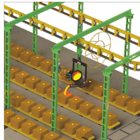
Monorail system for pouring
